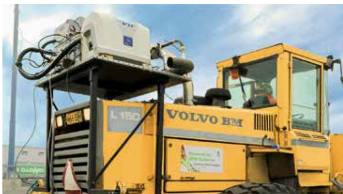
The recent test in Vuosaari Harbour focused on measuring the tailpipe emissions of a Volvo wheel loader construction vehicle
