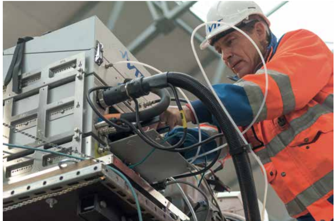
Lower particulate and nitrogen oxide emissions were noted in Vuosaari Harbour when VTT measured tailpipe emissions of renewable UPM BioVerno diesel in comparison to fossil diesel used in a Volvo wheel loader
