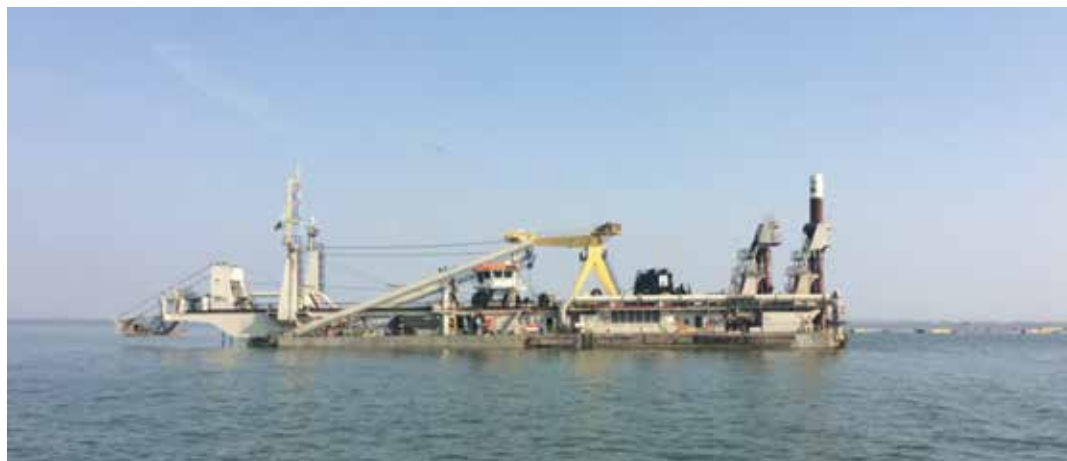
Boskalis vessel EDAX cutter suction dredger has successfully used biofuel in bio/fossil blends going up to 50%
